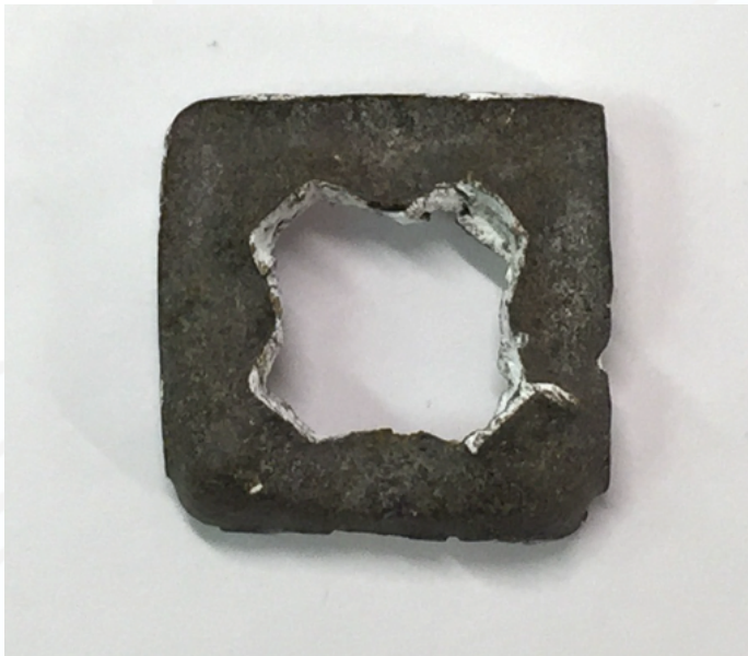
Regolith voxel shown is approximately 25mm by 25mm by 10 mm
